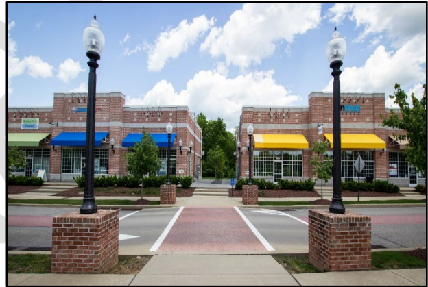
A series of shopfront and vertical variations to building facades are intended to promote a main street type of environment that de-emphasizes the horizontality of buildings.
